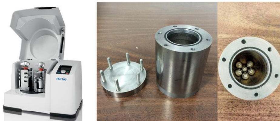
Figure 2.1 Photos of Retsch PM 200 planetary ball mill and grinding jars and balls
